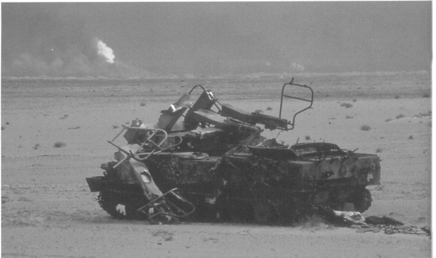
What is left of an SA-6 Gainful surface-to-air missile system near the Sabriya oilfield area. Each launcher vehicle carries 3 missiles which are guided by the Straight Flush radar system. The missile has a range of 4 to 22km and a maximum speed of Mach 4.
