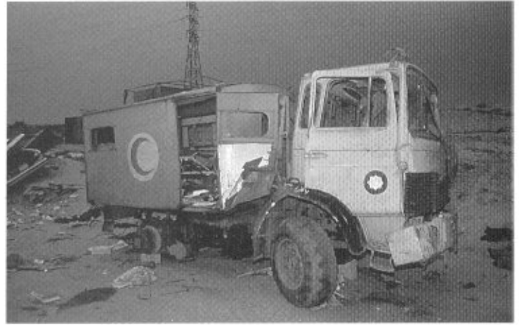
Iveco Magirus 75-13 AWM (4x4) 2,500kg truck (formerly Magirus-Deutz model 130M7FAL) in ambulance version. The former West Germany, like the former East Germany, sold a large number of trucks (4x4, 6x6) to Iraq.
