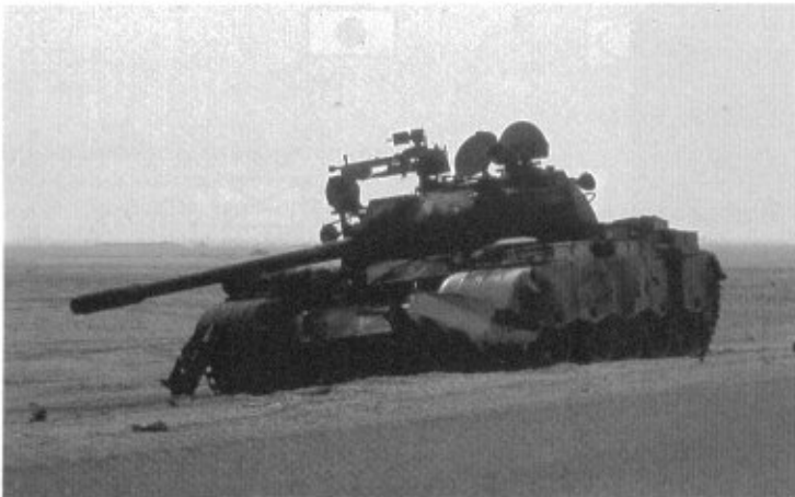
Victim of an A-10 Warthog, this T-55 has the KMT-6 mine plough attached and the 12.7mm machine gun still intact.
