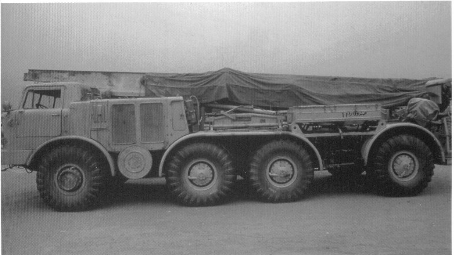
A BAZ-135L4 (8x8) chassis being used as tractor-erector-launcher (TEL) for FROG-7 (Free Rocket Over Ground 7) surface-to-surface tactical missile system. The warheads include nuclear, chemical, conventional high explosive, and cluster munition. Though Iraq did not possess nuclear warheads during the Gulf War, it had in service large quantities of chemical warheads.
