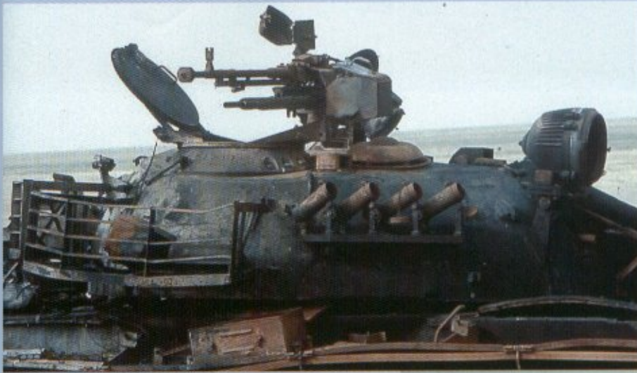
A Chinese-made T-69 knocked out by U.S. warplane. Note the laser rangefinder on the turret, above the 100mm gun.
