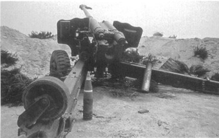
Iraqi 122mm field gun D-74s destroyed by Allied counter-battery. The D-74 was used primarily in support missions by the Iraqis. The D-74 has a maximum range of 24,000m and is operated by a crew of ten. It can be towed by the AT-L, AT-S, Ural-375D or the Tatra 813 tractors.
