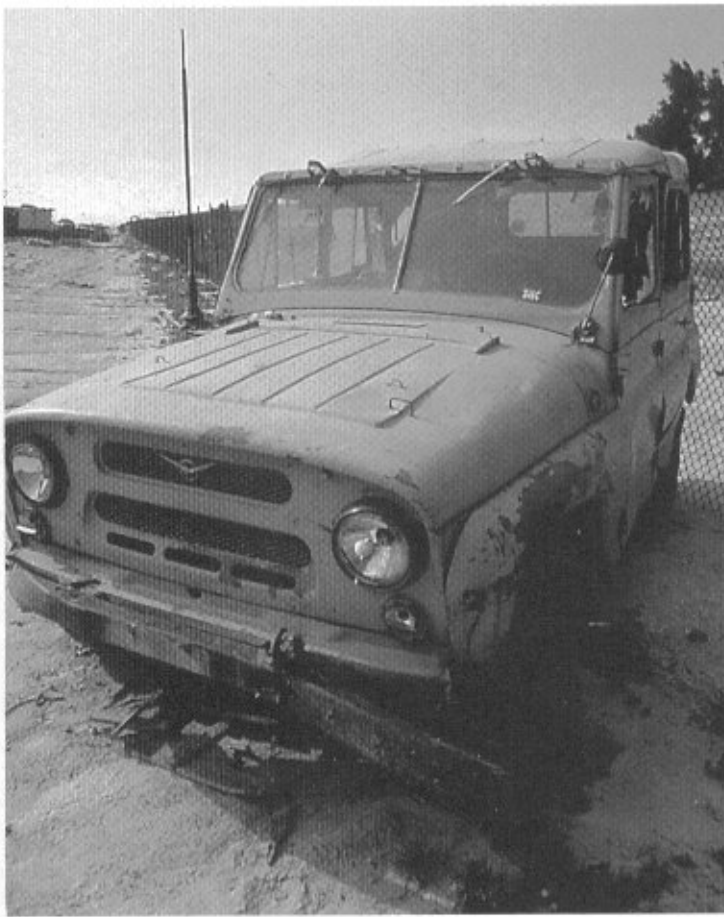
A Soviet-made UAZ-469B (4x4) 600kg jeep, a successor of the GAZ-69 jeep that equipped most of the former Warsaw Pact countries. The Iraqi army had thousands of this vehicle, and large quantity can be found abandoned in the desert in good conditions.
