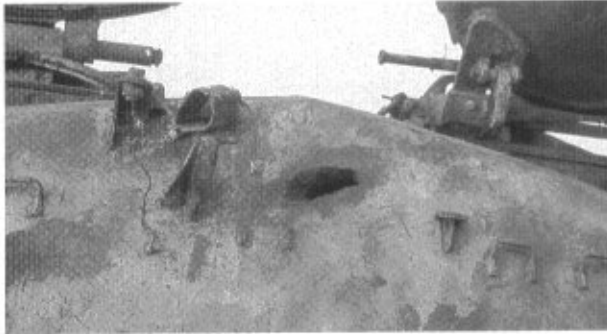
Effects of the A-10A gatling gun on T-55s and YW531. The 30mm projectiles can penetrate their armor easily.
