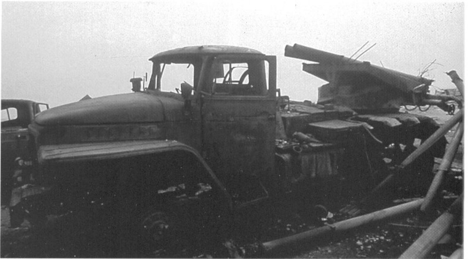
A burnt BM-21 multiple rocket launcher vehicle. The BM-21 consists of a standard Ural-375D (6x6) truck chassis fitted with a 40-round rocket launcher at the rear of the hull. The 122mm rockets can either be fired singularly or in a salvo.
