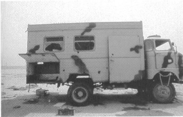
A shop-repair version of the LKW 6t truck. Note the special camouflage pattern.
