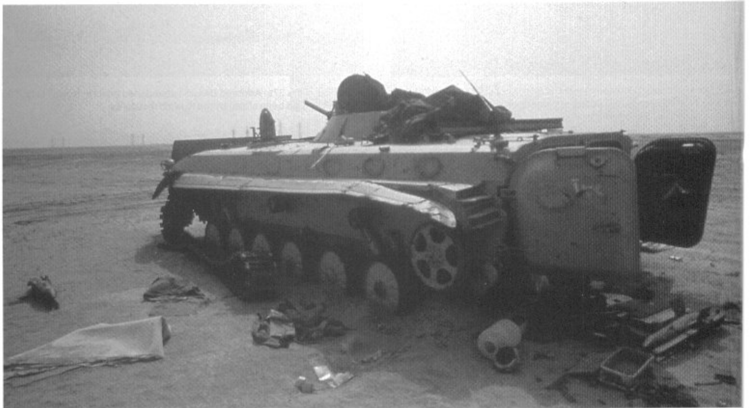
A BMP-1 infantry combat vehicle of a mechanized division near Sabriya oilfield. Before the Gulf War, Iraq had around 1,500 BMP-1/2. Since only the Republican Guard units employed BMP-2s, the BMPs found in Kuwait theatre were mainly BMP-1s. This BMP-1 lost a track during a tight turn while trying to escape and the crew had to abandon the vehicle. AT-3 Sagger missiles and 73mm shells were all over the place.
