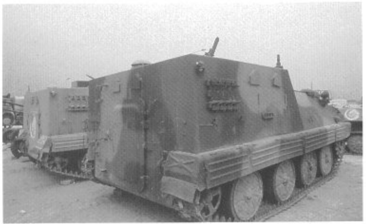
A Type YW701 command post vehicle and a Type YW750 armored ambulance captured by the French.
