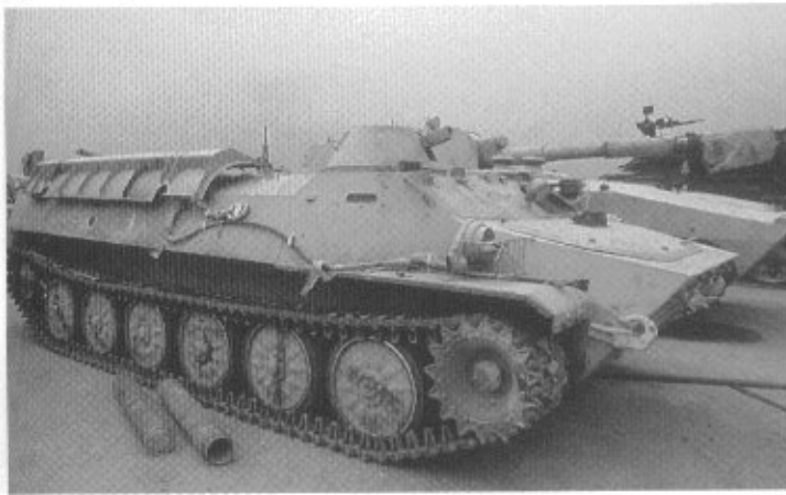
MT-LB engineer vehicle with a plough blade mounted on the roof.
