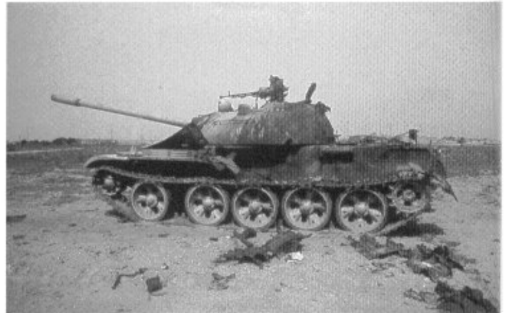
A T-55 of the 10th Armored Division received a hit at the bottom of the turret.
