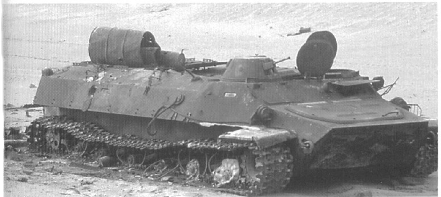
The Iraqi army left behind in Kuwait more than 50% of its fleet of 1,500 MT-LB multi-purpose tracked vehicle. Most of the units in Kuwait were equipped with this type of cheap armored personnel carrier and artillery tractor. The MT-LB, with its low ground pressure, has good cross country performance on soft sand.
