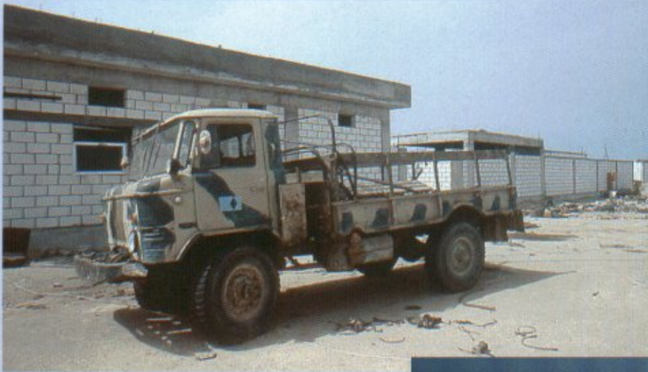
A Romanian-made LKW 6t truck (4x2) deserted by its crew. This is a different version of the TV-51 having a maximum road speed of 100km/h.
