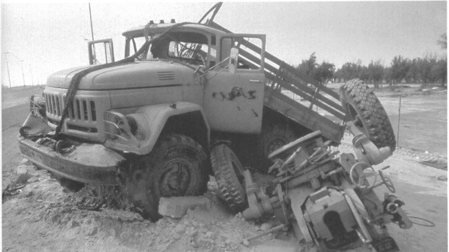
The ZIL-131 (6x6) 3,500kg truck was used by the Iraqis for transporting cargo, personnel and as the tractor for towed artillery such as the 122mm D-30 howitzer. Here, a ZIL-131 truck and a D-30 artillery destroyed along a highway leading away from Kuwait City.
