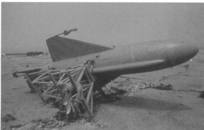
SS-N-2 Styx anti-ship missiles found on a naval base south of Kuwait City. This missile equipped the Osa class missile boats.
