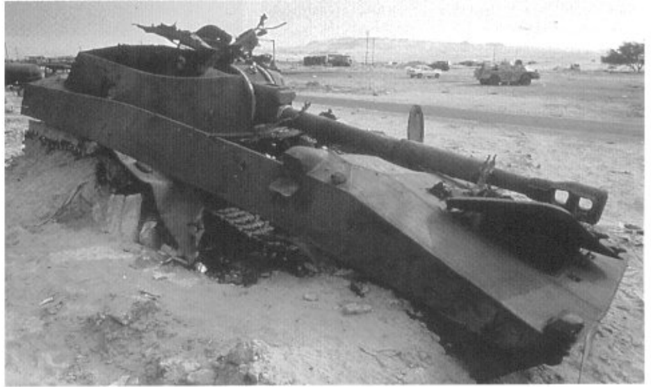
2S1 Gvozdika 122mm self-propelled howitzer is built on an extended MT-LB chassis. The main armament is a modified version of the 122mm D-30 towed howitzer. It has a rate of fire of 5 rounds per minute and the 2S1 normally carries 40 122mm projectiles.
