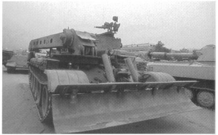
An IMR (Inzhenernaia Mashina Razgrazhdeniia) combat engineer vehicle captured in good condition by the French Army. The IMR is an engineer vehicle for obstacle-clearing based on the T-55 chassis.
