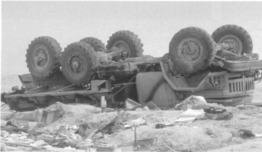
A burnt BM-21 multiple rocket launcher vehicle. The BM-21 consists of a standard Ural-375D (6x6) truck chassis fitted with a 40-round rocket launcher at the rear of the hull. The 122mm rockets can either be fired singularly or in a salvo.
