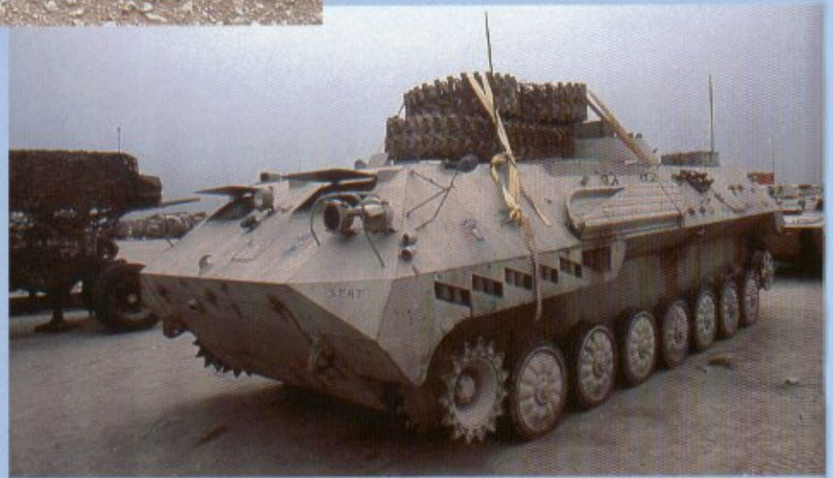
ACRV (Artillery Command and Reconnaissance Vehicle) minus its tracks. These vehicles were assigned to Iraqi 2S1 and 2S3 self-propelled artillery batteries as battery fire direction center and command vehicles.
