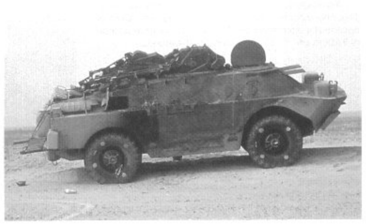
A burned down SA-9 Gaskin mobile surface-to-air missile system. The SA-9 has a maximum range of 7,000m with altitude limits being 900 to 5,000m.
