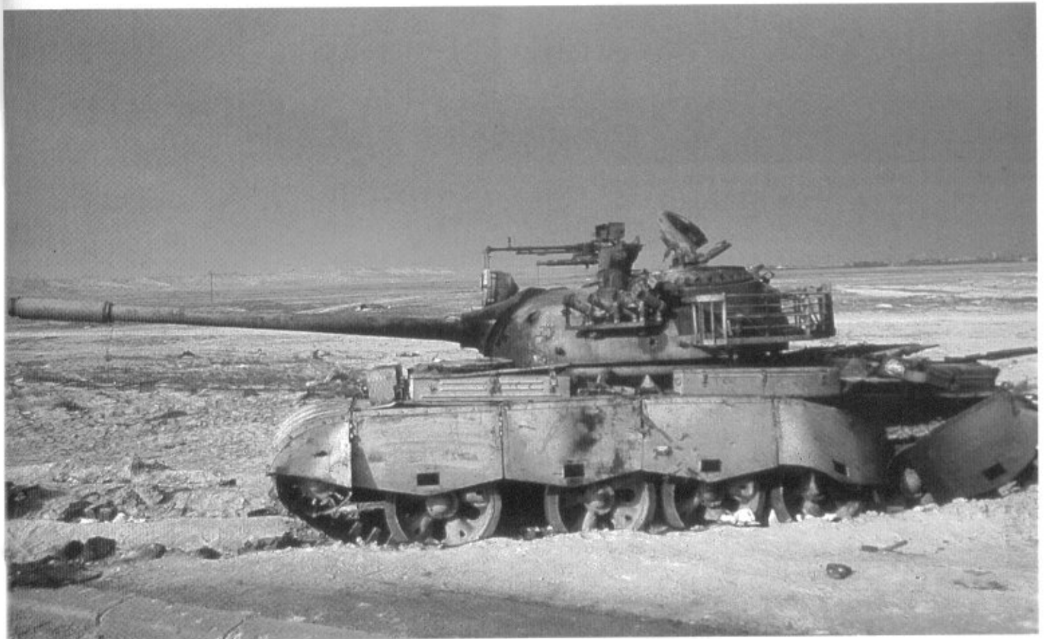
A Chinese-made T-59 tank of the 6th Armored Division fitted with side skirts, that was knocked out by the U.S. 7th Corps west of Kuwait. Notice the penetration on the lower side of the turret.
