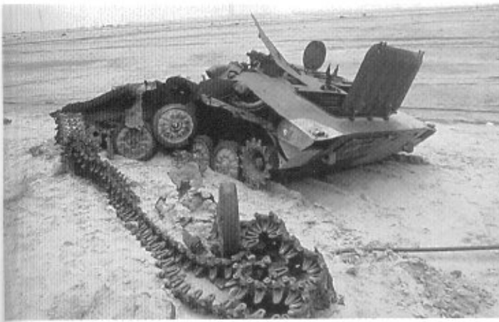
2S1 Gvozdika 122mm self-propelled howitzer is built on an extended MT-LB chassis. The main armament is a modified version of the 122mm D-30 towed howitzer. It has a rate of fire of 5 rounds per minute and the 2S1 normally carries 40 122mm projectiles.
