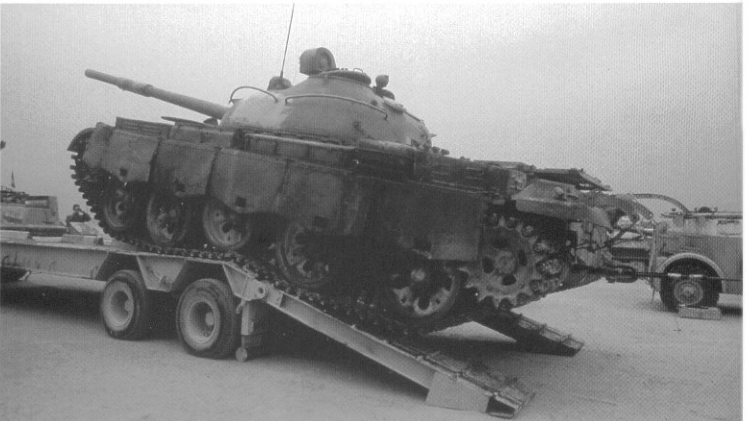
A captured T-62 dismantling from a French Army trailer. Notice the Panhard M3/VAT repair vehicle in the background.
