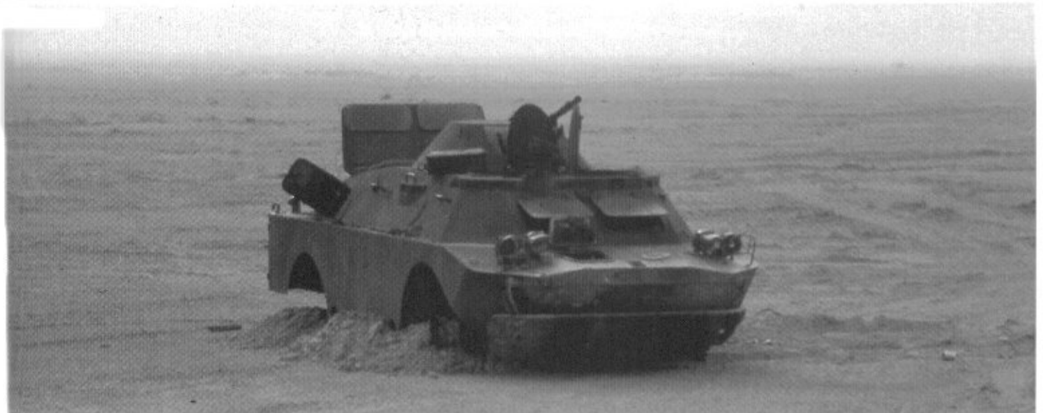
A BRDM-2 wreck destroyed at Umm Al Aish. This amphibious scout car has a turret mounting a 14.5mm KPVT machine gun with a coaxial 7.62mm PKY machine gun.
