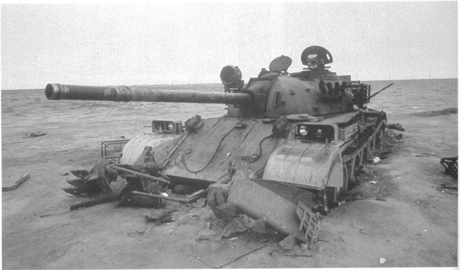
This T-59 with KMT-6 mine plough of the 1st Mechanized Division seen near the Al Birgan oilfield.
