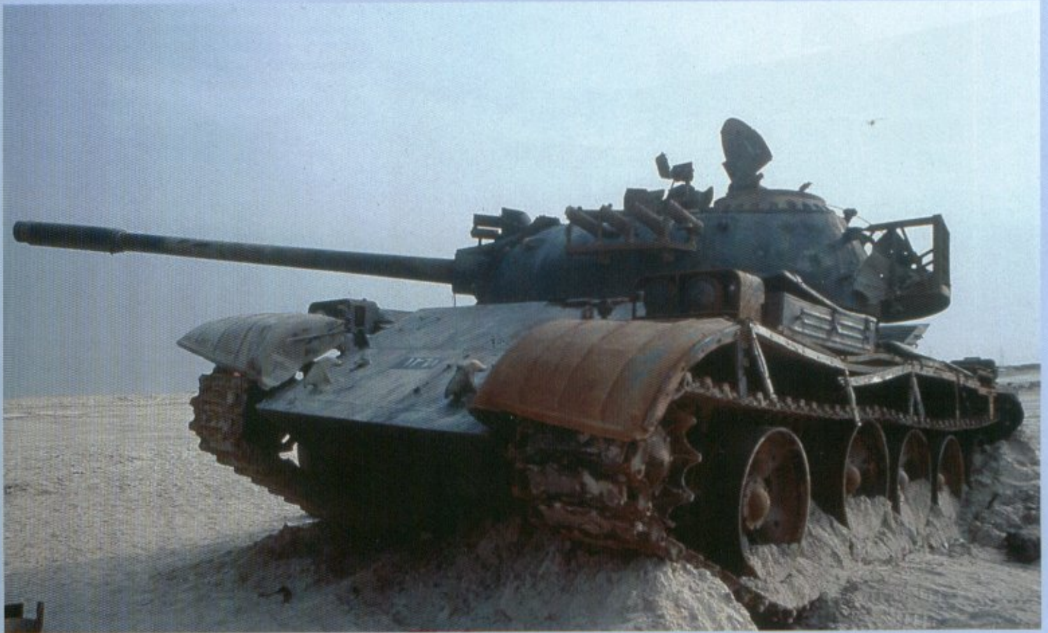
A Chinese-made T-69 knocked out by U.S. warplane. Note the laser rangefinder on the turret, above the 100mm gun.
