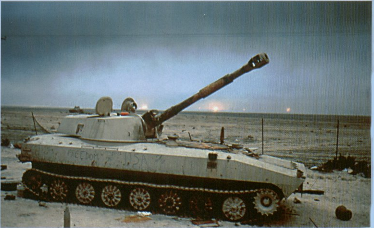
A Soviet-built 122mm 2S1 self-propelled howitzer of the 1st Mechanized Division disabled near the Al Birgan oilfield. (SIRPA)
