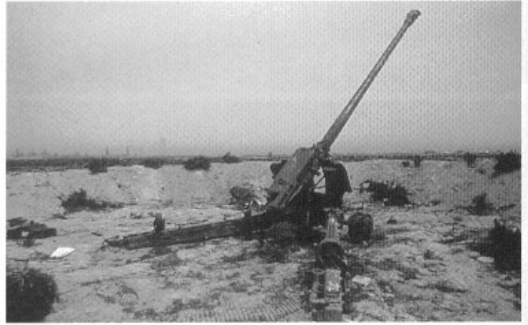
Iraqi 122mm field gun D-74s destroyed by Allied counter-battery. The D-74 was used primarily in support missions by the Iraqis. The D-74 has a maximum range of 24,000m and is operated by a crew of ten. It can be towed by the AT-L, AT-S, Ural-375D or the Tatra 813 tractors.
