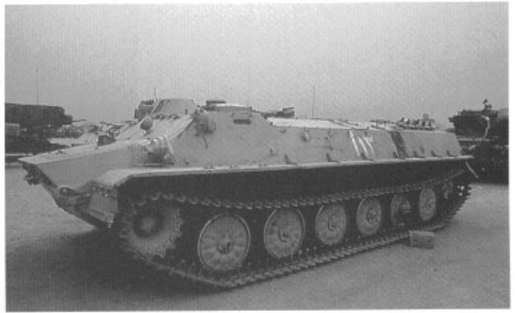
MT-LB multi-purpose tracked vehicle in armored personnel carrier configuration.
