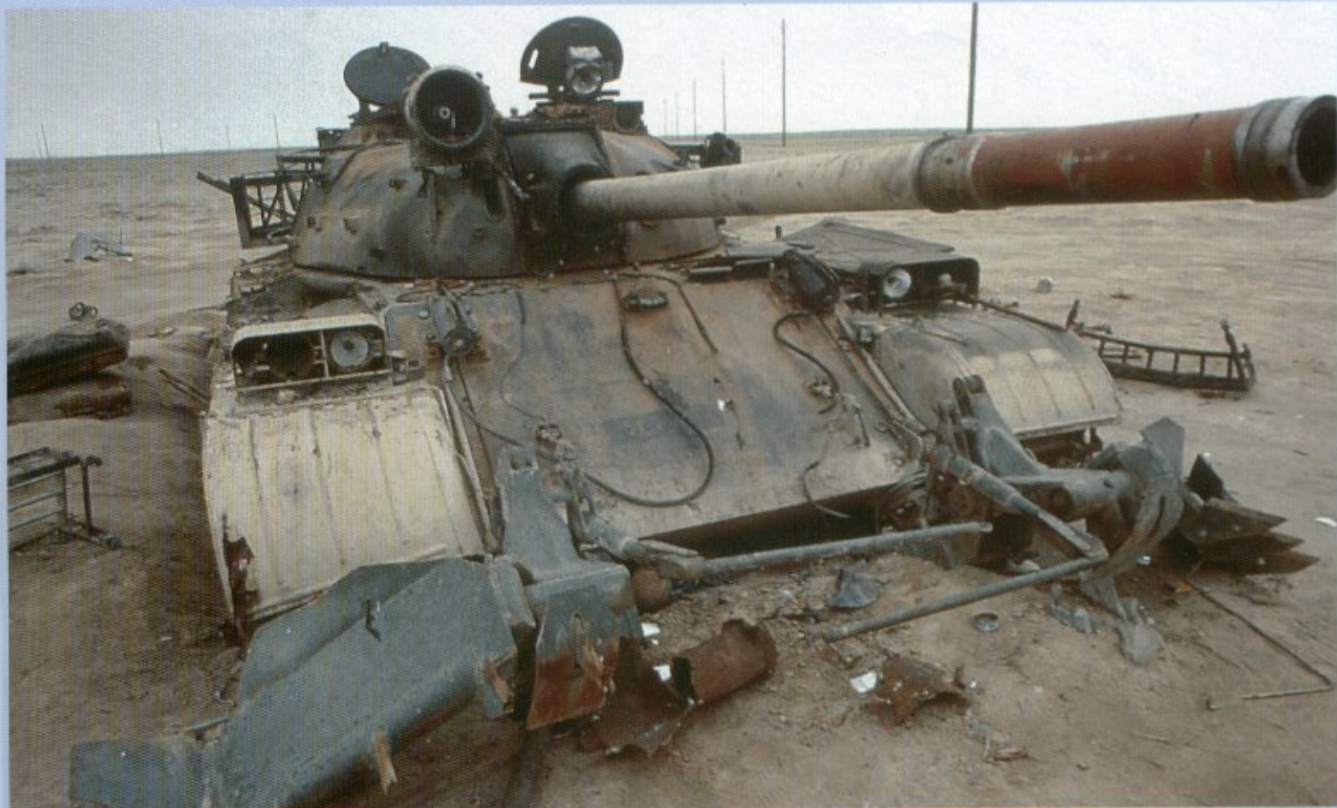
A destroyed T-59 near the Al Birgan oilfield area. This T-59 is fitted with the KMT-6 mine plough and belonged to an assault engineer company of the 1st Mechanized Division.
