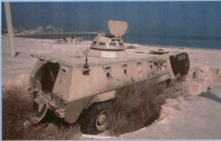
An Egyptian manufactured FAHD armored personnel carrier captured by the Iraqis and turned into a mobile pillbox guarding the water-front in Kuwait City. This FAHD was designed by Thyssen Henschel with a French Creusot-Loire TLI turret, and armed with twin 7.62mm machine guns. The FAHD is amphibious and can carry twelve infantrymen plus a crew of two.
