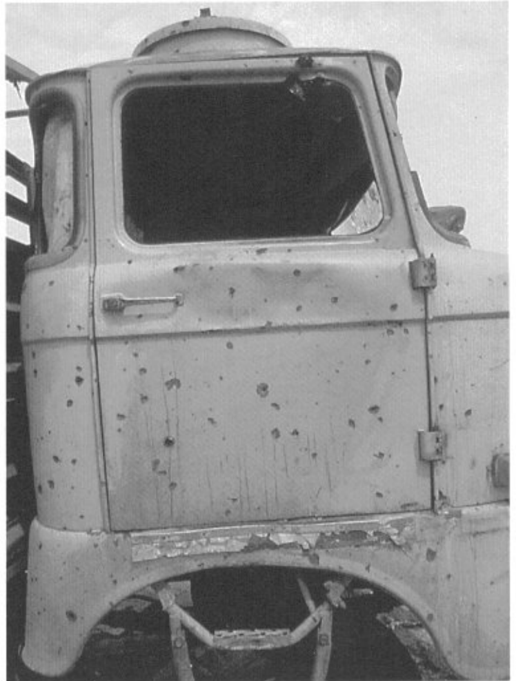
GAZ-66 truck hit by sub-munitions of a U.S. cluster bomb.
