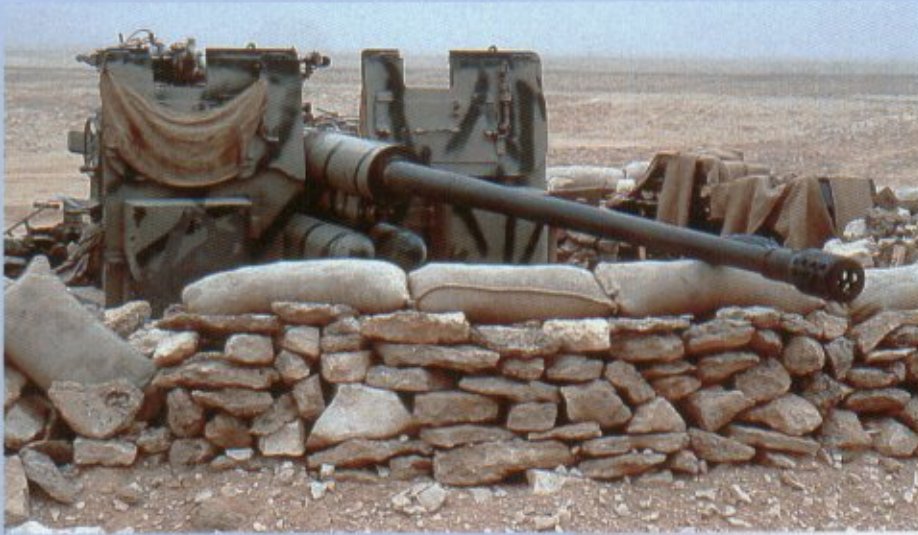
ACRV (Artillery Command and Reconnaissance Vehicle) minus its tracks. These vehicles were assigned to Iraqi 2S1 and 2S3 self-propelled artillery batteries as battery fire direction center and command vehicles.
