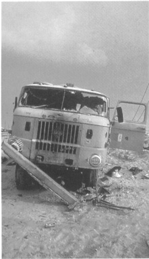
Destroyed W50LA/A (4x4) 3,000kg truck used by the majority of Iraqi divisions for general transport purpose. The W50L series of trucks were manufactured in former East Germany. It has a maximum road speed of 83km/h and a range of 720km.
