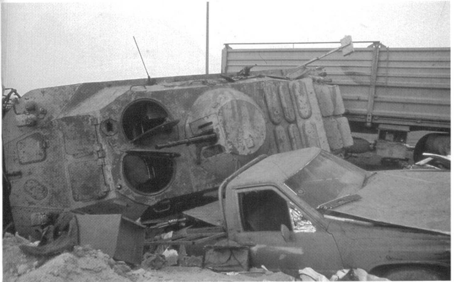
One of the many victims at Multa Gap, a BRDM-2 equipped with a 14.5mm KPVT machine gun in the turret. Notice the Toyota pick-up underneath the BRDM.
